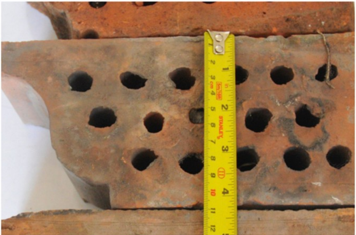
Reclaimed Brick Corbels Sourced To Match Original Damaged Bricks
